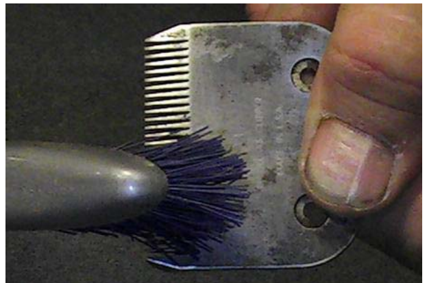
Brushing the rust from between the blade teeth on both cutter and comb.
